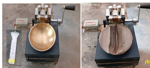
Figure 4. Casagrande dish.
