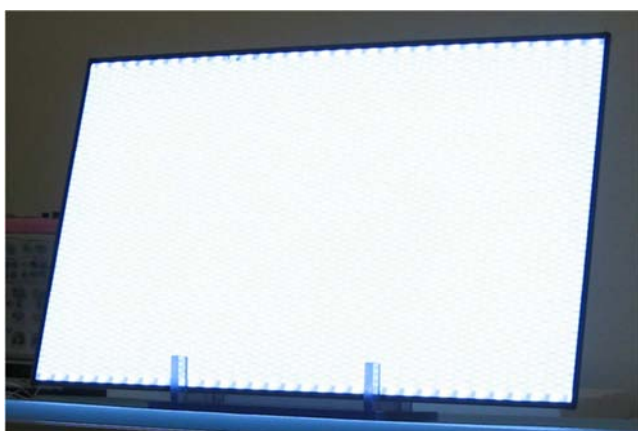
Figure 10. Lighted flat panel that contains 4 coil-EEFL lamps in the vacuum-sealed panel container.
