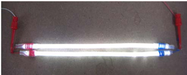
Figure 6. Two lighted coil-EEFL lamps in parallel connection under DC voltage at 4 kV.
