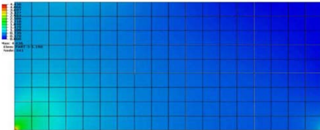
Figure 42. Stresses in Unreinforced Masonry Wall (Mpa) subjected to a uniformly distributed load of 800KN/M 2 .
