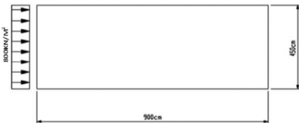
Figure 19. Load Case 3: 800KN/M2 Uniformly Distributed Load Applied to Unstrengthened Masonry Wall.
