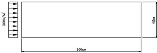
Figure 16. Load Case 2: 600KN/M2 Uniformly Distributed Load Applied to Unstrengthened Masonry Wall.
