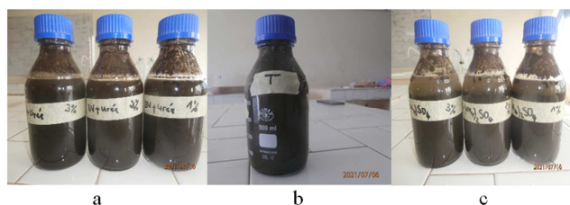
Figure 1. Treatment reactors: a. urea; b. no additive; c. ammonium sulphate.
