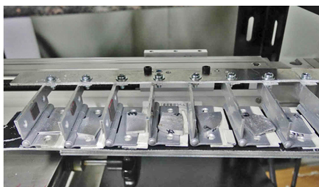
Figure 6. Aluminum alloy samples set in the sequential sample cells.
