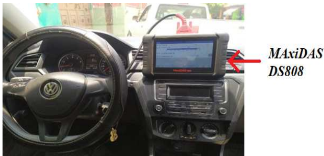
Figure 1. MaxiDAS808 oscilloscope scanner connected to the car.
