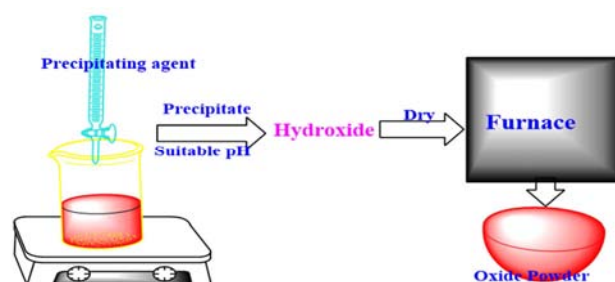
Figure 6. Synthesis of photonanocatalyst by co-precipitation method.
