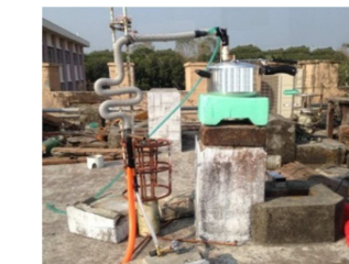
Figure 3. Arrangement of pyrolysis unit.
