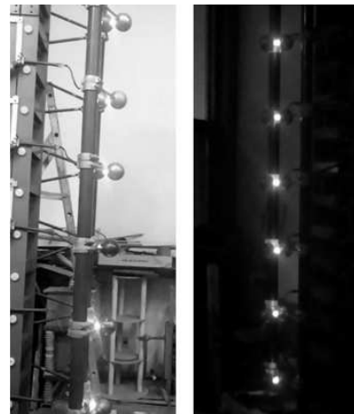
Figure 18. Experimental IVG triggering and the discharge of its capacitors.
