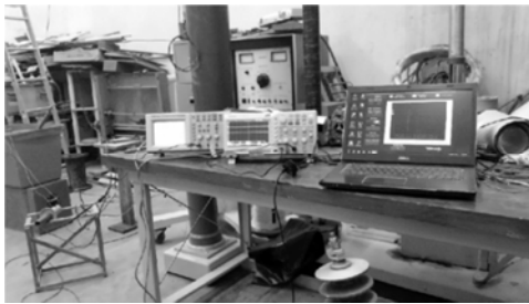
Figure 15. Impulse voltage measurement with a high-voltage probe.
