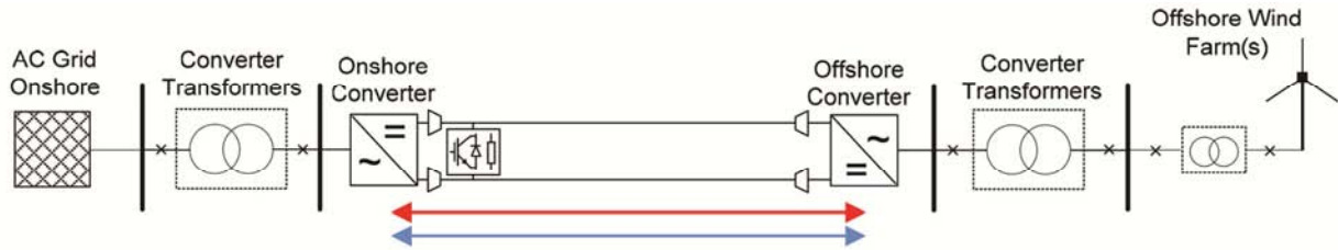
Figure 8. Grid connection of offshore wind farm through VSC HVDC transmission system.
