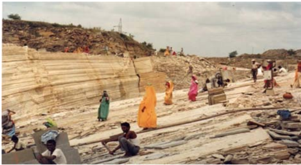
Figure 8. Manual Mining with High Bench Heights.
