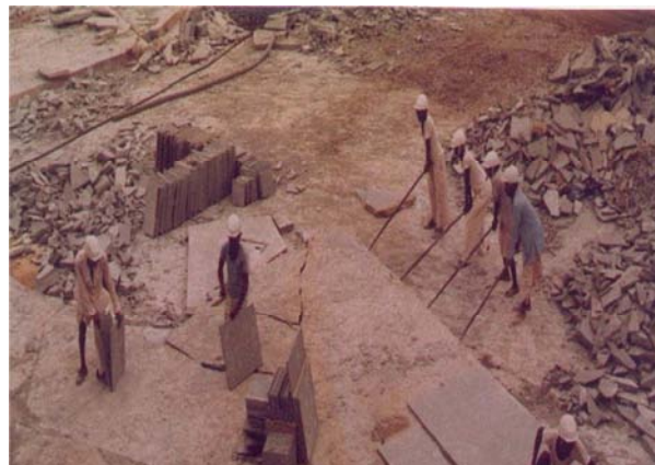
Figure 2. Manual Quarrying of Kotah Stone.
