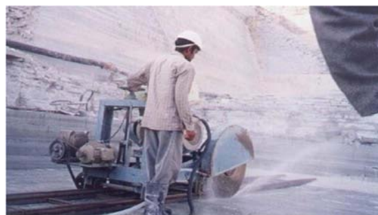
Figure 7. Cooling Water Ejecting out in form of Mist.
