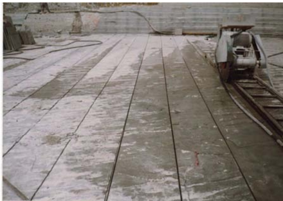
Figure 5. Jhiri Machine Cutting Kotah Stone Layers at 2 ft interval.
