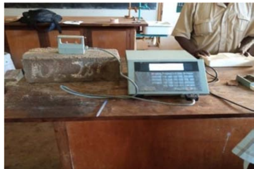
Figure 2. Determination of thermal conductivity of the blocks.
