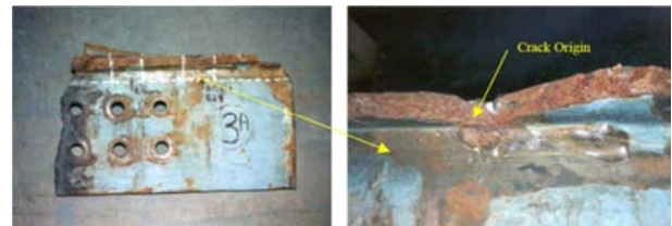
Figure 6. Hoan Bridge fracture initiation [15].
