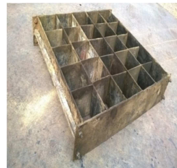
Figure 1. 100 mm x 100 mm cast tray used in producing the test cubes.
