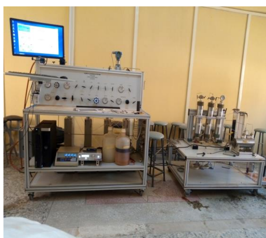
Figure 4. Core-flooding experimental set-up.
