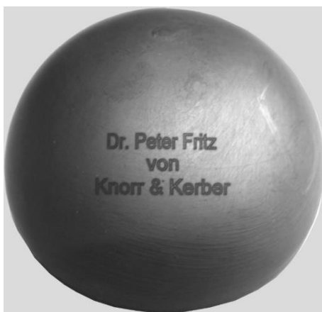
Figure 4. Laser engraving: permanent traceability for nuclear material control [7].
