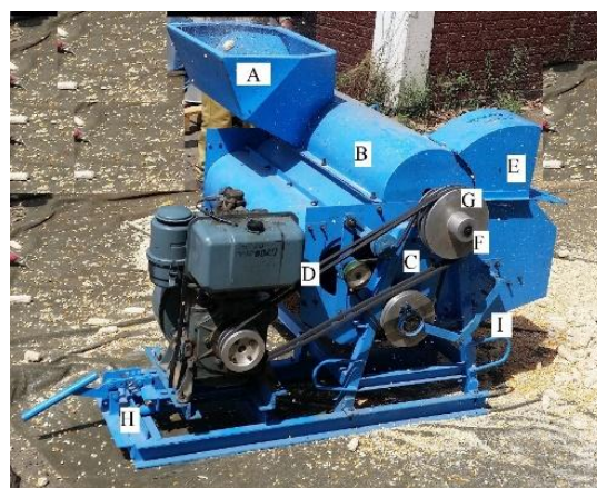
Figure 1. Melkassa developed engine driven maize Sheller.
