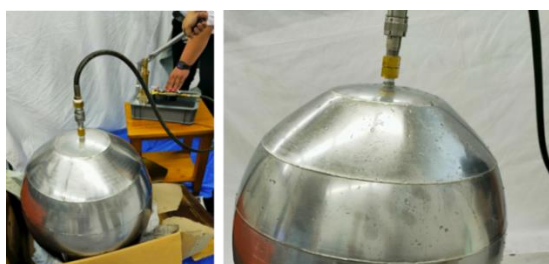
Figure 11. Forming egg-shaped laminated shell structure by internal.
