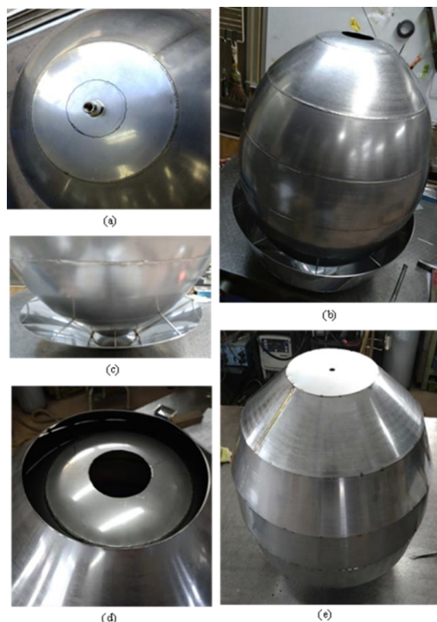
Figure 9. Fabrication of the middle layer connecting rods and the egg-shaped outer shell.
