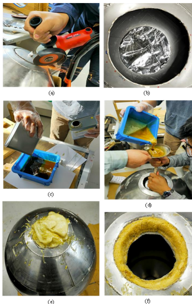
Figure 12. Manufacturing process of egg-shaped laminated tsunami shelter structure.
