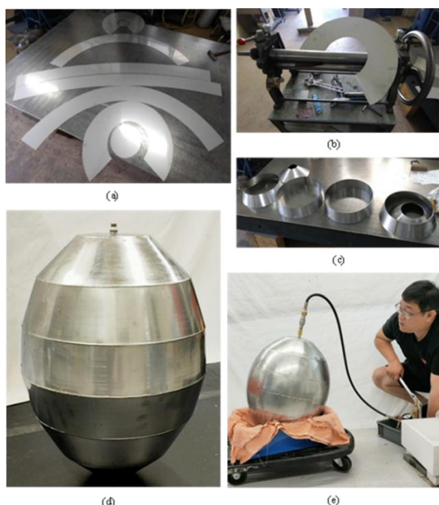
Figure 8. Fabrication of the inner shell of a laminated egg-shaped shell.
