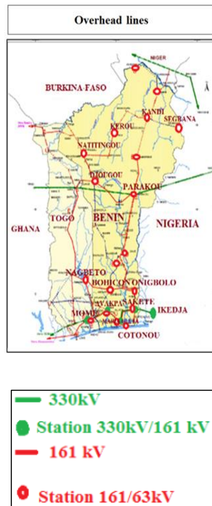
Figure 1. Configuration of high-voltage B transmission lines in Benin [17].
