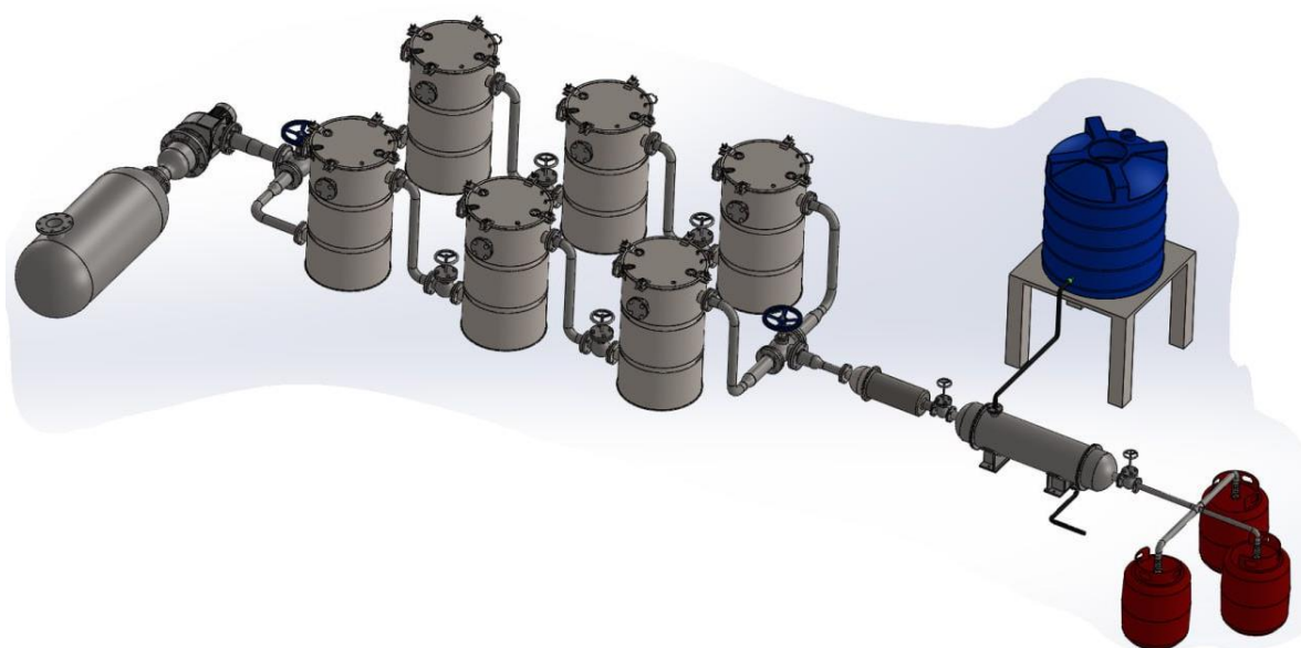
Figure 2. Mechanical Design Assemble of Effluent Flue Gas Used for Charcoal Production.
