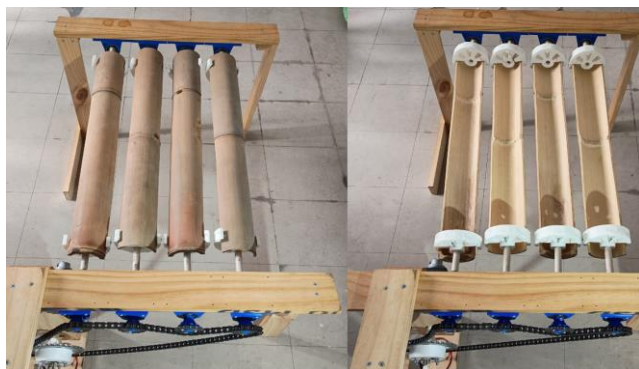
Figure 4. Scale rainwater harvesting prototype to capture rainwater (left: standby mode; right: collection mode).
