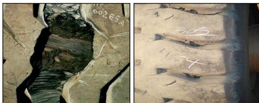
Figure 14. Haul Truck Tyre Separation.
