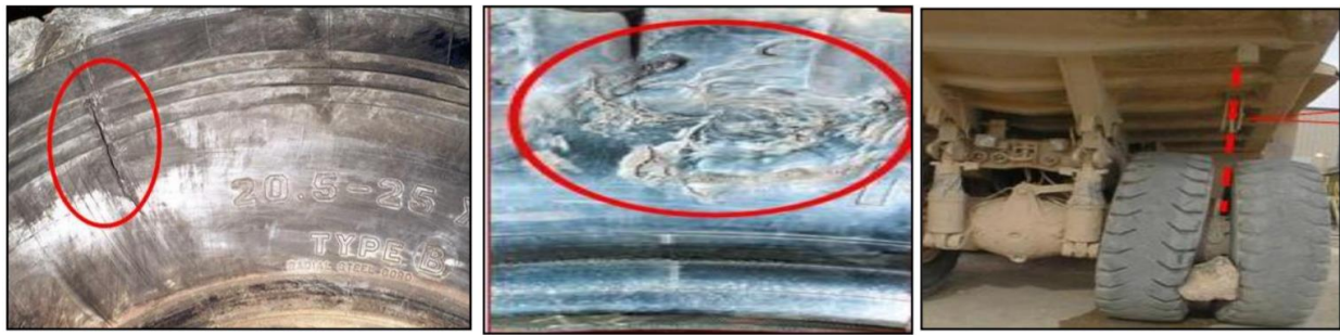
Figure 6. Haul Truck Tyre Sidewall Cut.
