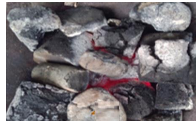
Figure 8. Briquettes made from banana peels.
