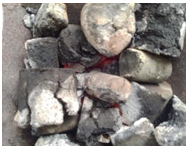
Figure 10. Briquettes made from orange peels.
