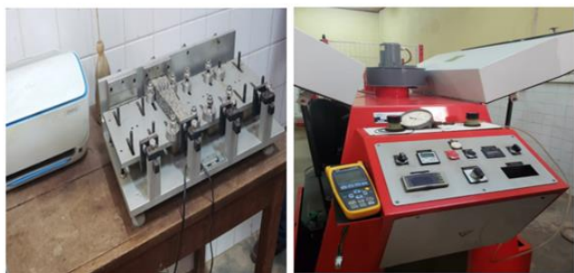
Figure 11. Stiffness test in the trapezoidal bituminous specimens in the laboratory.
