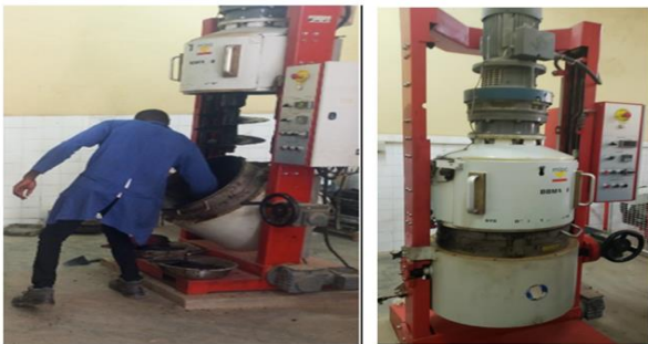
Figure 6. Testing the bituminous concrete specimen on the gyratory shear press.
