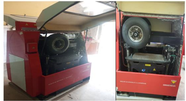
Figure 7. Rutting test machine and tests on the bituminous slab.
