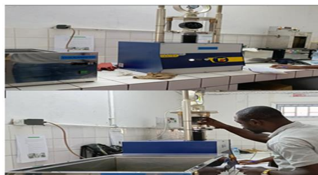
Figure 10. ITSr Stability Test of BBEM3 with 0.3% CECABASE 300 Dosage.
