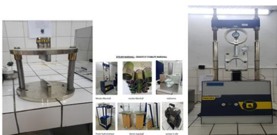
Figure 8. Bituminous specimens and Marshall test of BBEM3 with 0.3% CECABASE 300 Dosage.
