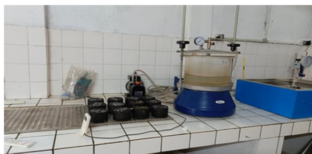
Figure 9. ITSr Tests of BBEM3 with 0.3% CECABASE 300 Dosage.
