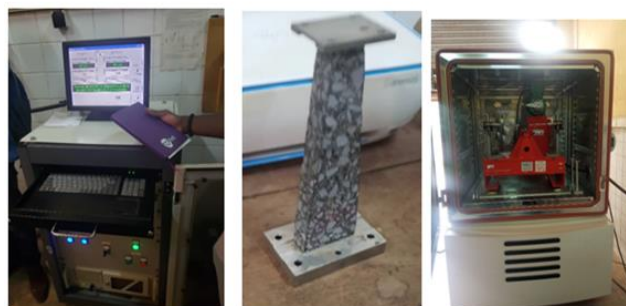
Figure 12. Fatigue test performed on trapezoidal bituminous specimens.
