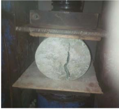
Figure 3. Tensile splitting strength test.
