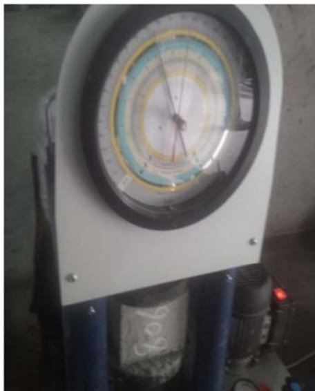
Figure 1. Compression strength test machine.
