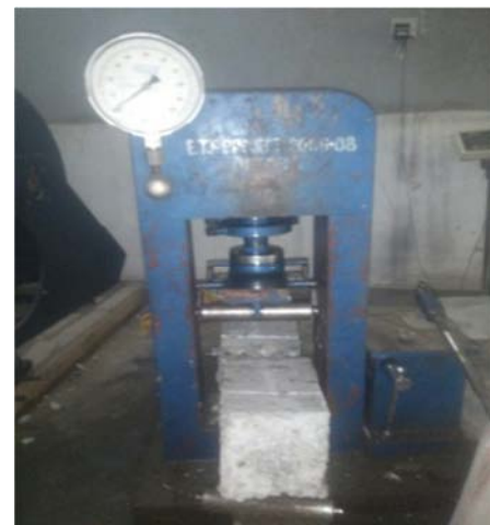
Figure 2. Flexural strength test machine.
