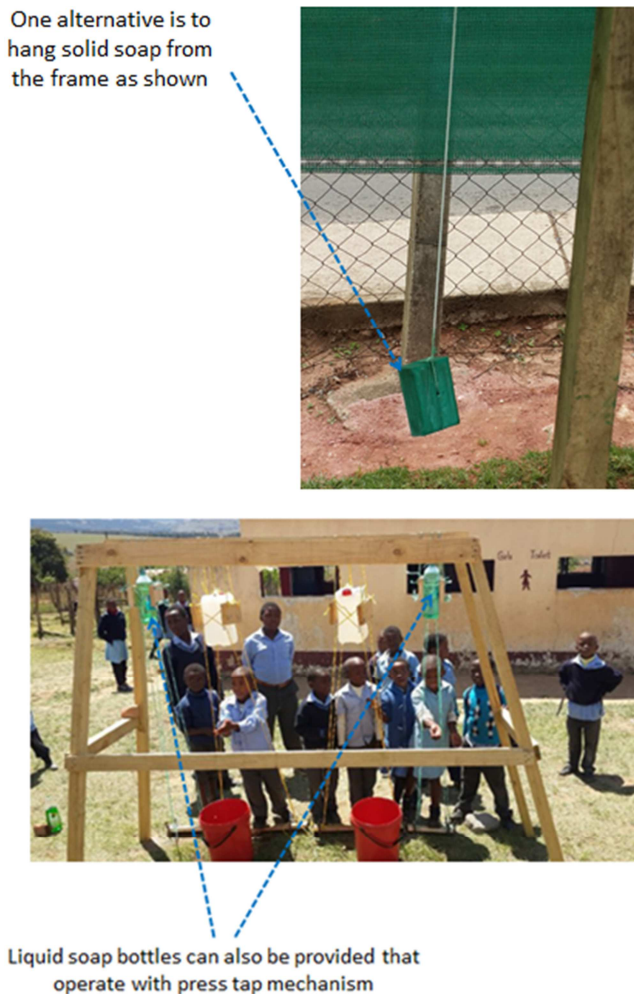
Figure 12. Alternative provision for soap: Solid soap tied with string from the supporting frame and liquid soap that operated on the same principle of a Press Tap.
