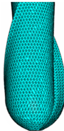
Fig. 11. Initial mesh of the ball end mill model.
