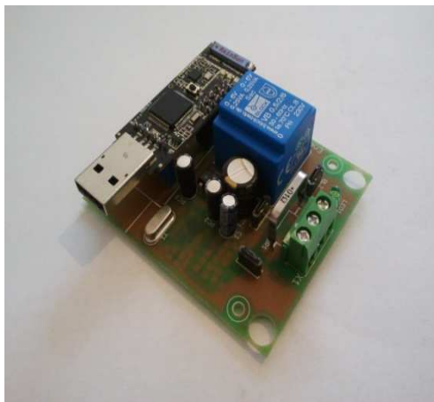
Figure 5. Electric sensor used as a relay node.
