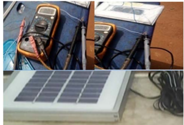
Figure 6. The multimeter side by side with the fabricated solar module and a prototype conventional solar module as testing was in progress.
