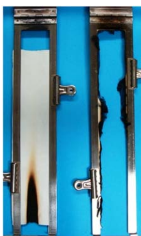
Figure 5. Picture of treated twill fabric (15.7 % add-on, left) and untreated control twill fabric (0 % add-on, right) after vertical flammability test by ASTM D-6413-11 method.
