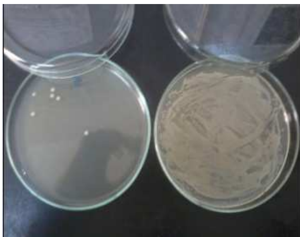
Figure 7. Contact test result for E. coli after 24 hrs incubation. The right plate represents the negative control plate. The left plate represents the count after contact with PAN loaded with Ag NPs for 18 hours.
