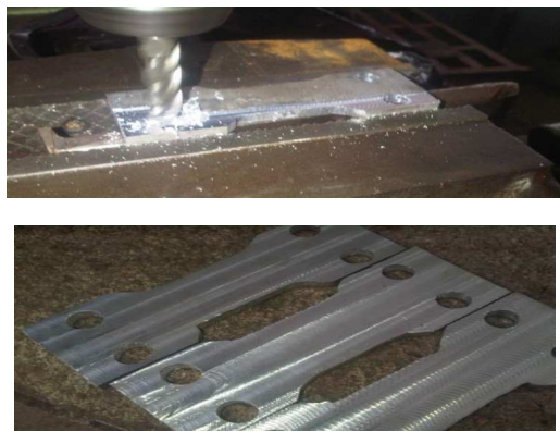
Figure 2 (a) and (b). Drilling holes into specimen to be subjected to end milling; Specimen which have been subjected to end milling
