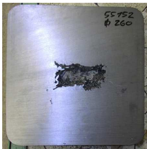
Figure 1. Transverse cut of the hot-rolled billet made from 34CrMo4 steel with internal defect.
