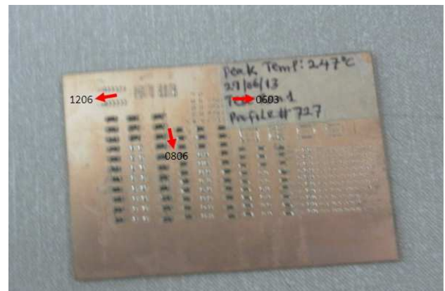
Figure 1. Copper board with an array of 1206, 0806 and 0603 chip resistors
