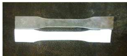
Figure 1. The shape of the tensile test specimen.
