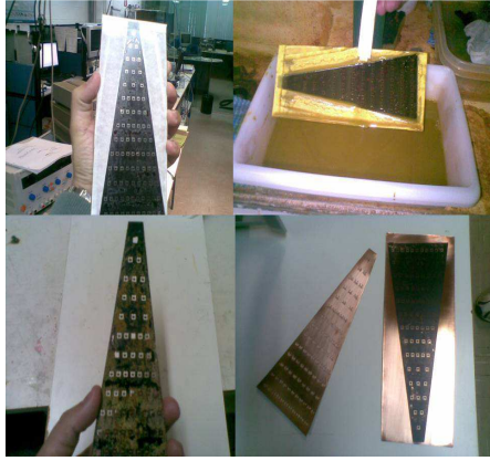
Fig. 20. Septum fabrication on a cooper foil under etching and finished.
