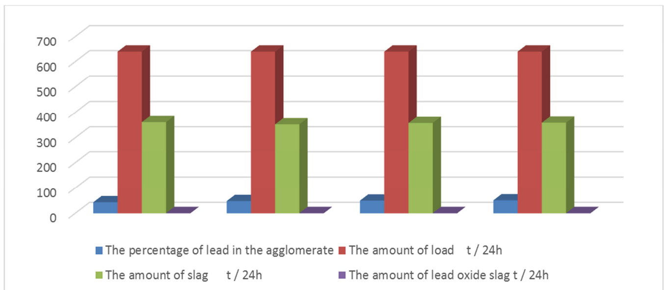
Fig. 4. Percentage of Lead agglomeration and its impact on the amount of oxide Lead slag. 6. Conclusions.
