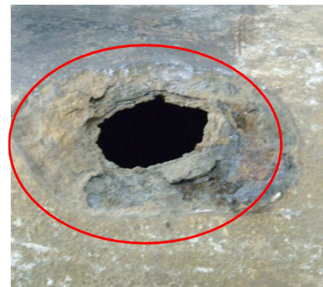
(g) Corrosion perforation defect; effective zone 35 mm, relative mesh dimension 12 mm
