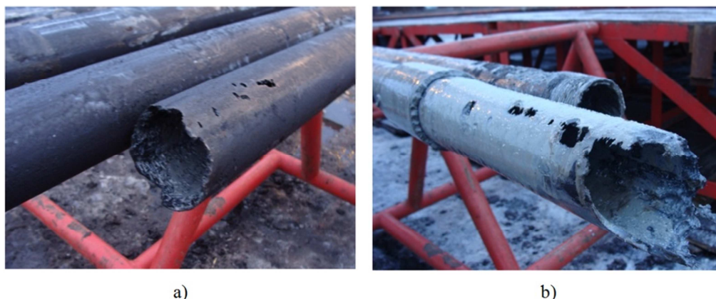
Figure 1. The general view of the typical tubing pipe corrosion damages (a, b) resulting of operation condensate fields by private corporation “Naftohazvidobuvannya”, Ukraine.
