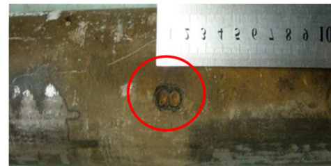
(e) local corrosion cavities of size 8 mm, depth 1,8 mm
