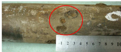
(b) local corrosion cavities, full depth 3,2 mm
