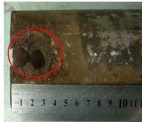
(f) corrosion perforation defect of length 40 mm
