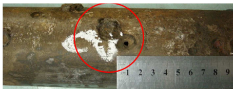
(c) local corrosion cavities with perforation defect diameter 3 mm
