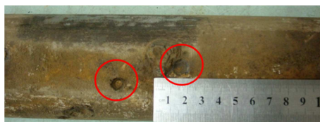
(d) local corrosion cavities of size 8 and 12, full depth 2 mm
