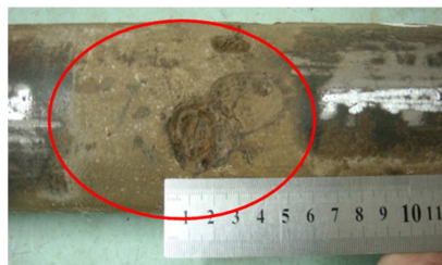
(a) local corrosion cavity, full depth 3 mm
