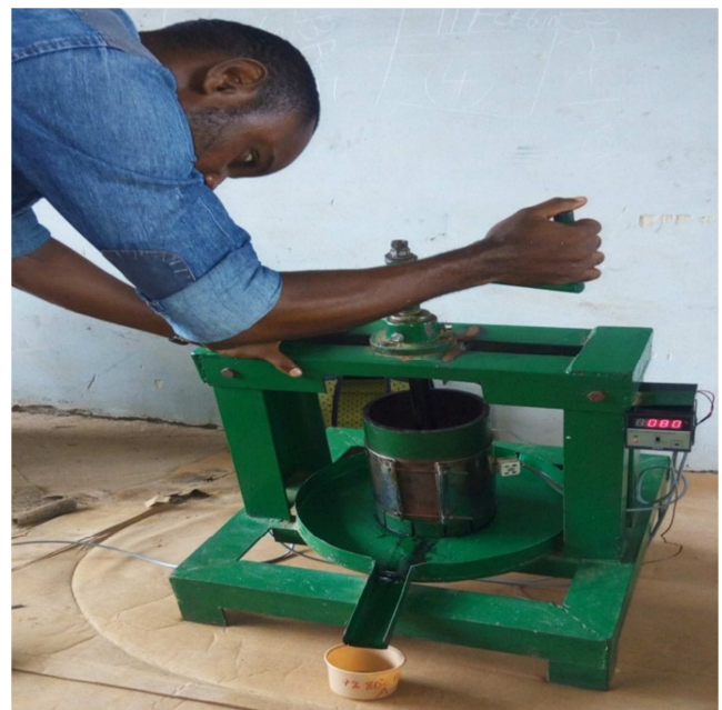
Figure 1. Pictorial view of the screw press during pressing operation.
