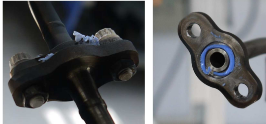
Figure 4. Structure of B-end after test.
