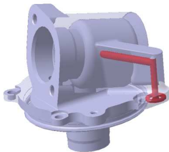
Figure 13. Design change of blind pipe.
