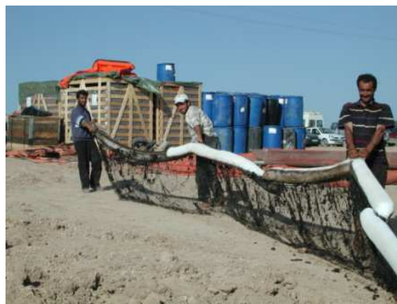
Figure 19. The fishnetted boom prepared for oil collection, [11] and [12].
