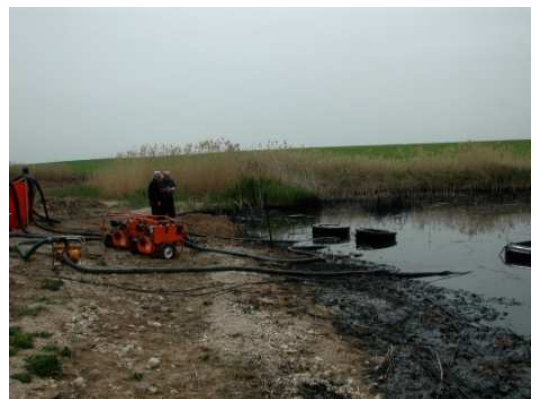
Figure 15. Working skimmer on the oily shoreline, [11] and [12].
