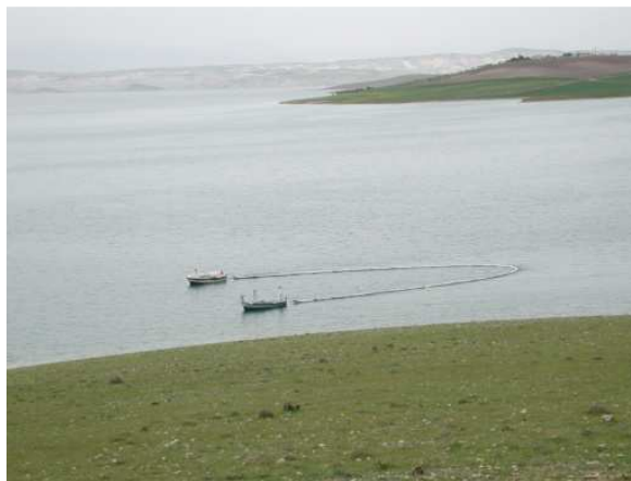
Figure 21. A fishnetted boom in oil recovery from the lake waters, [11] and [12].
