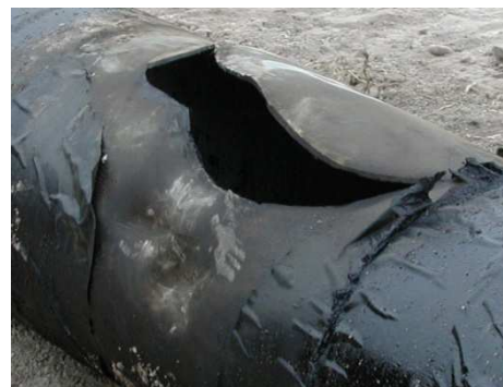
Figure 1. Ruptured pipeline, [11] and [12].
