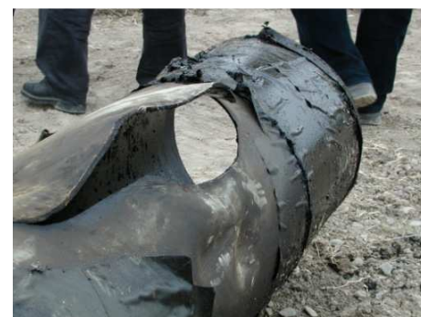
Figure 2. Another view of ruptured pipeline, [11] and [12].
