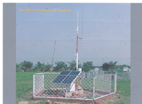
Figure 3. Installed Lightning detector in Bangladesh.
