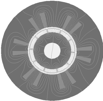
5 pairs of poles, 6 main teeth and radial trapezoidal wave-form structure
