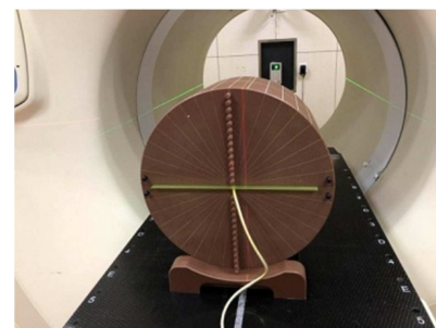
Figure 2. Setup of rotational output dose detection.
