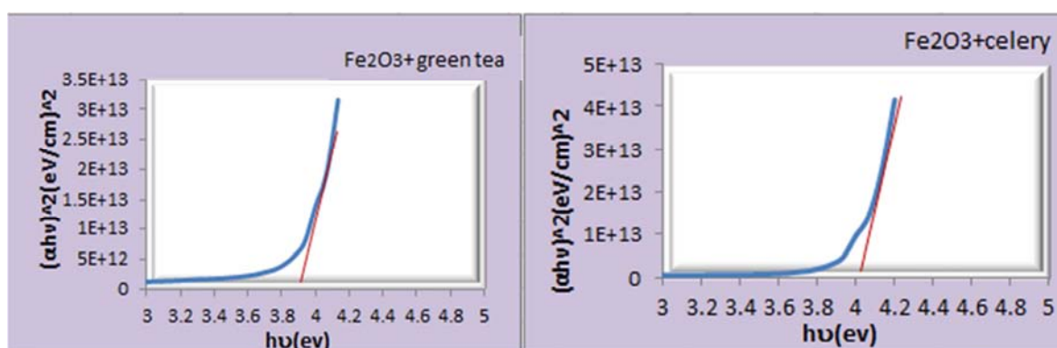
Figure 7. The energy band gap of Iron oxide Nanoparticles with Camellia sinensis extract and Apium graveolens extract.
