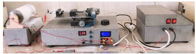
Figure 3. Homemade electric spinning device.
