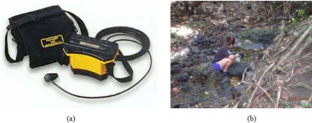
Figure 5. (a) Marsh-McBirney “Flow-Mate” flow meter; and (b) Research assistant installing a level logger in Toguan river.
