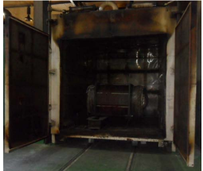
Figure 3. HV motor in drying oven.
