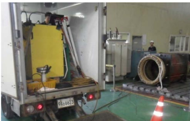
Figure 2. Insulation diagnosis test.
