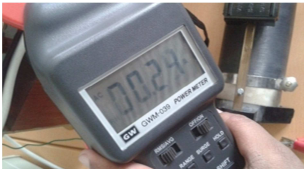
Fig. 5. Current reading using a clamp meter.
