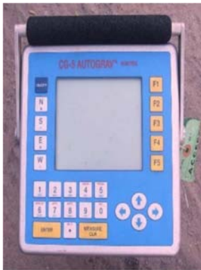
Figure 5. CG-5 Autograv utilized for gravity data acquisition.
